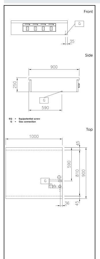
Gas Gas Power: 34 kW Gas Type Option: Gas Inlet: 1/2" **Key Information:** External dimensions, Width: 1000 mm External dimensions, Depth: 900 mm External dimensions, Height: 250 mm Net weight: 82 kg Configuration: One-Side Operated;Top Front Burners Power: 8.5 - 8.5 kW **Back Burners Power:** 8.5 - 8.5 kW **Back Burners Dimension -**Ø 70 Ø 70 Front Burners Dimension -
